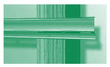
The resilient channel is attached to the wall studs before sheetrock is applied. It decreases noise levels by dampening vibrations. Absorptive insulation should also be installed in the air cavity to prevent an amplification of sound within the wall.
